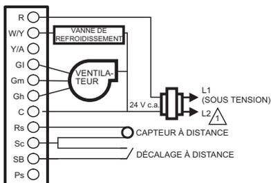
⚠ ALIMENTATION. ASSURER AU BESOIN UN DISPOSITIF DE COUPEURE ET UNE PROTECTION CONTRE LES SURCHARGES.
