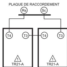
⚠ LE TR21-A EST UN CAPTEUR DE 10 K OHMS.
