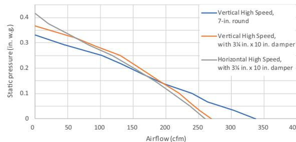
HVI-2100 CERTIFIED RATINGS comply with new testing technologies and procedures prescribed by the Home Ventilating Institute, for off-the-shelf products, as they are available to consumers. Product performance is rated at 0.1 and 0.25 in. static pressure at high speed based on tests conducted in an HVI-approved state-of-the-art test laboratory. Sones are a measure of humanly-perceived loudness, based on laboratory measurements.
