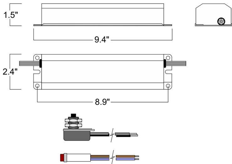
A test switch and charging indicator light are provided.
