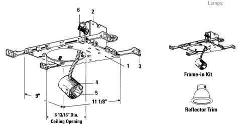
Complete Fixture consists of Reflector Trim & Frame-In Kit. Select each separately.
