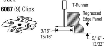
Slotted Grid Ceilings such as Donn Finline and Chicago Metallic Ultraline 3500 and 3600. Use two per 2' and 4' track, three per 8', and four per 12' track.
