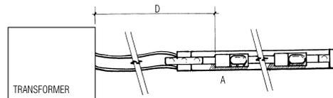
$$\text{VOLTAGE DROP} = 2D \times A \times \Omega$$
