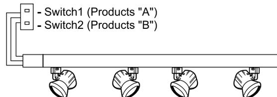
Where wattage requirements are 2400W or more the trac run may be fed from one point, providing 4800W capacity plus 2 switches.
