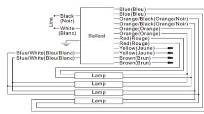
For five lamp operation, individually cap yellow leads. Insulate to 600Volts
