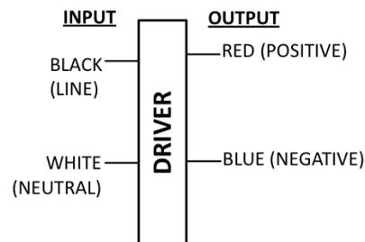
Input and output use lead wires.
